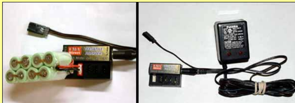
Left: An 8-cell, 600mAh NiMH pack plugged into an FMA universal adapter, which is plugged into a radio system charger (transmitter side).
